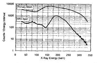
Figure 3. Energy spectrum recorded during a transmission diffraction experiment on a 6 mm thick nickel alloy (N5) single crystal casting in a mold (5 mm wall thickness). X-ray parameters were 320 kV, 0.75 mA. A 25 mm thick lead collimator, with a 2 mm clear aperture was placed on the 37 mm diameter x 13 mm thick intrinsic Ge detector to separately sample the two spectra by centering the aperture on the primary beam or the diffraction spot.
