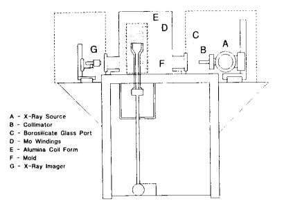
Figure 4. Resistively heated directional solidification furnace, fitted with a collimated x-ray source and real timexray imager for transmission x-ray diffraction studies during casting of single crystal nickel superalloys.
