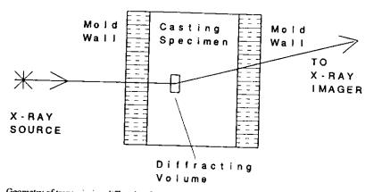
Figure 1. Geometry of transmission diffraction from a crystalline specimen surrounded by a casting mold.
