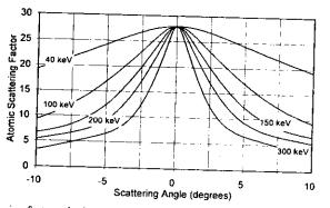
Figure 2. Atomic scattering factor calculated for nickel, plotted as a function of scattering angle for several x-ray energies.
