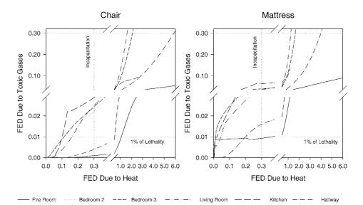
Figure 7. Comparison of incapacitation from thermal effects and narcotic gas effects for two single item fires in a ranch house.
