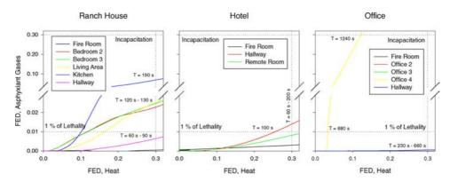
Figure 4. Comparison of thermal effects and narcotic gas effects for several different geometries.
