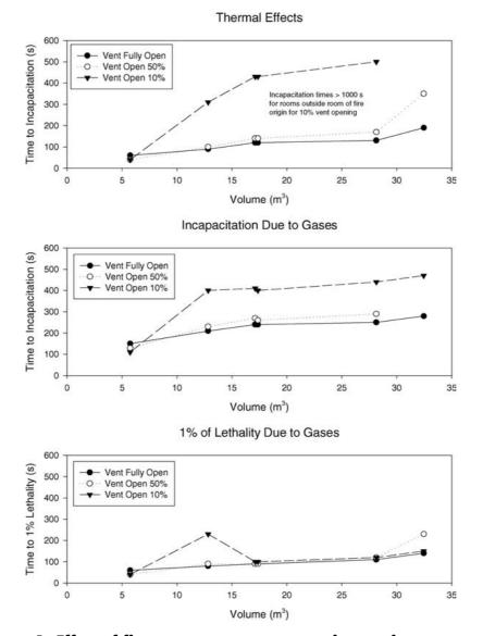
Figure 6. Effect of fire compartment vent opening on time to incapacitation due to thermal and narcotic gas effects for several rooms in a ranch house.
