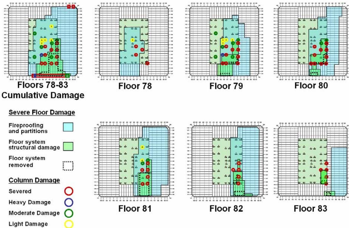
Figure 7–3. Calculated damage to floors 78 through 83 in WTC 2 (see NIST NCSTAR 1-6).
