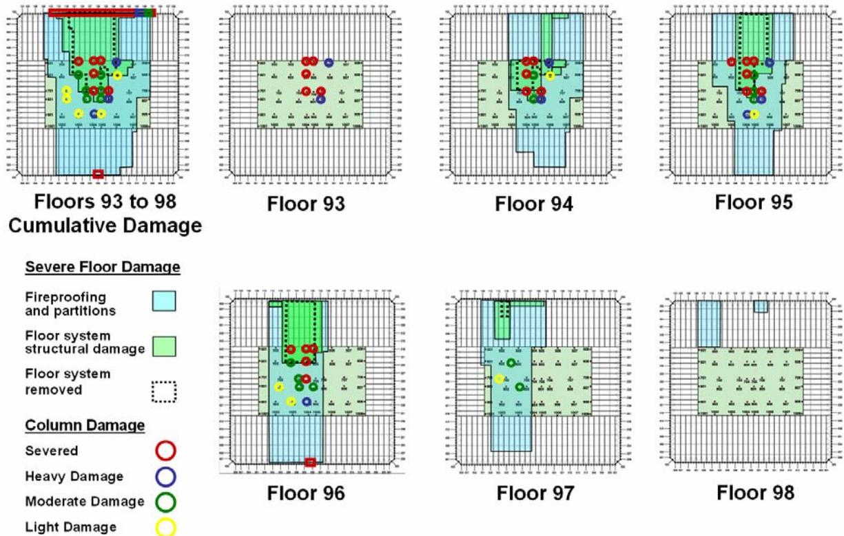
Figure 5-3. Calculated damage to floors 93 through 98 in WTC 1.
