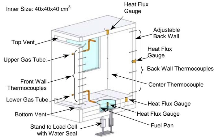
Fig. 1. Schematic half-view of the experimental configuration.
