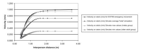
Figure 6. Comparison of velocity vs interperson distance on stairs using EXIT89 and Simulex for 'hotel' simulation.
