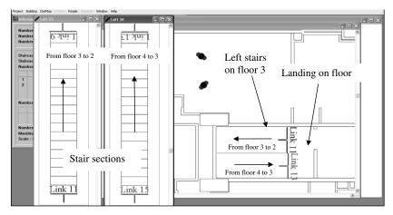
Figure 3. Separate stair configuration in Simulex.
