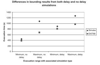
Figure 7. Comparison of evacuation results (times) using EXIT89 and Simulex for the performance-based design simulations.
