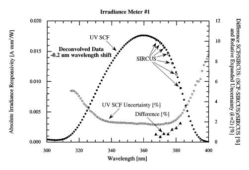
Fig. 4. Plot of irradiance responsivity, UV SCF relative expanded (k = 2) uncertainties, and relative differences for the two methods for irradiance meter #1. Irradiance meter #1 is a typical commercial 365-nm detector with an  $\approx$ 50-nm bandpass (FWHM).
