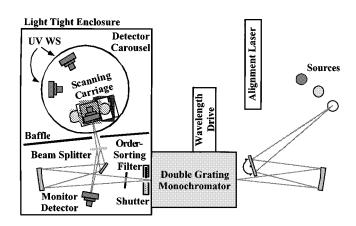
Fig. 1. UV SCF diagram. The irradiance meter-under-test is mounted on the scanning carriage. Spectral-responsivity comparison is accomplished by rotating the detector carousel to place one of the UV working standards (WS) into the beam. The order-sorting filter removes second-order light beyond 400 nm.
