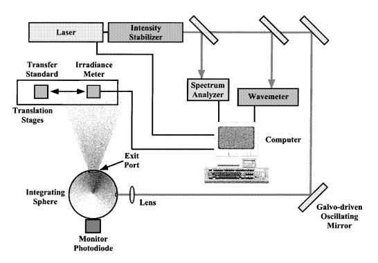
Fig. 2. SIRCUS diagram. The irradiance meter calibration is performed by direct substitution with the irradiance transfer standard.
