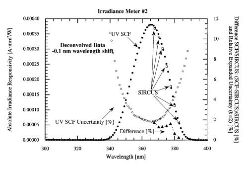
Fig. 5. Plot of irradiance responsivity, UV SCF relative expanded (k = 2) uncertainties, and relative differences for the two methods for irradiance meter #2. Irradiance meter #2 is a NIST designed transfer standard with a  $\approx$ 25-nm bandpass (FWHM).
