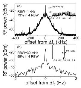
Fig. 1. Heterodyne beat measured around 900 nm between the two FLFCs with  $\Delta f_0 = 101$  MHz. (a) Measurement with a RF spectrum analyzer at 1-kHz RBW. Inset, measurement with 1-Hz RBW. (b) Measurement of the beat mixed to 10 Hz with a fast Fourier transform spectrum analyzer at 30-mHz RBW (inset, with 3-mHz RBW, linear scale). The fraction of overall power contained in the central peaks is indicated.
