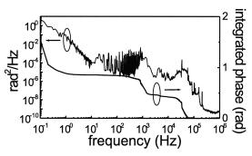
Fig. 2. Left-hand axis, phase-noise power spectral density of the  $\Delta f_0$  beat, equivalent to the phase noise of the optical frequency comb components around 900 nm (333 THz). Right-hand axis, integrated phase noise.
