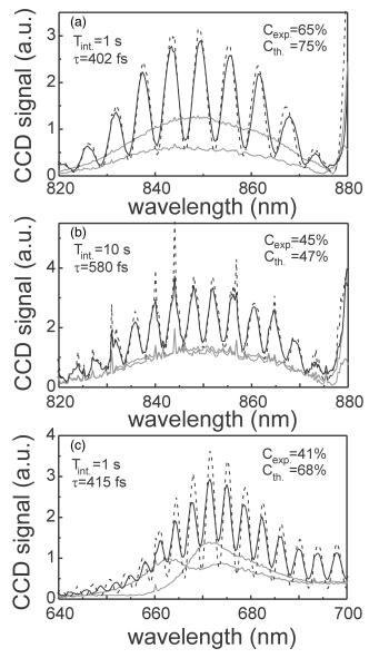
Fig. 3. SIs (solid black curves) between NIST-BB1 and NIST-BB2, the individual laser spectra (solid gray curves), and theoretical SIs calculated from the individual spectra (dashed curves): (a) using the infrared output of the FLFCs and  $T_{\rm int.} = 1$  s, (b) same as (a) with  $T_{\rm int.} = 10$  s, (c) using the visible output and  $T_{\rm int.} = 1$  s. The pulse spacing  $\tau$  and the experimental and theoretical contrast are also indicated.
