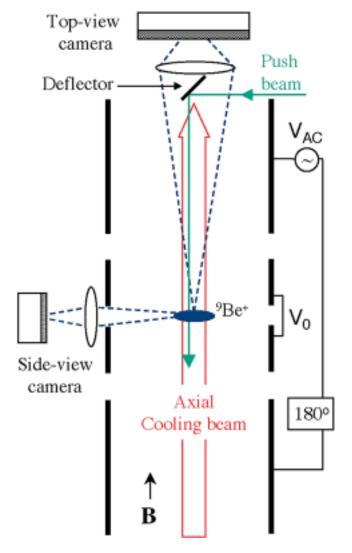
Fig. 1. The cylindrical experimental apparatus and its optical diagnostics. In this work B = 4.46 T and  $V_0$  ranged from -1 kV to -2 kV.
