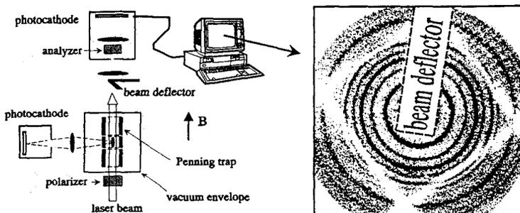
Figure 1. Apparatus and Bragg scattering image from  ${}^9\text{Be}^+$  ions in a Penning trap.
