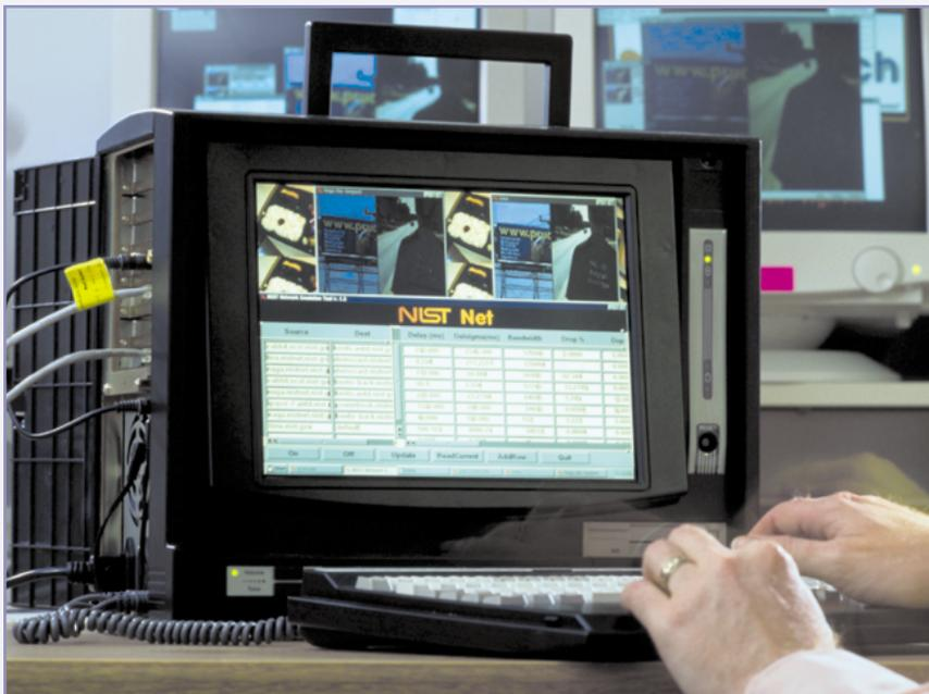
*NIST Net allows controlled, reproducible experiments with QoS-sensitive Internet applications and protocols to study the effect of Internet performance dynamics on adaptive video applications.*
