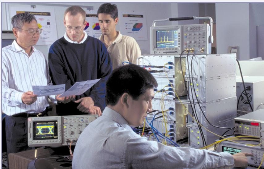
*J. Wen monitors the performance of the Wavelength Division Multiplexing (WDM) network equipment. D. Su (left), E. Hagley, and F. Lapeyrere examine the test results. The WDM equipment was developed for metrology of optical networks.*
