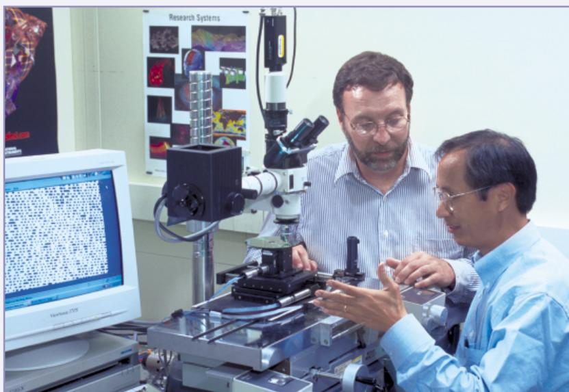
*F. Byers and X. Tang test reliability of a digital versatile disc (DVD). Digital information stored on the DVD can be seen on the screen through a microscope.*
