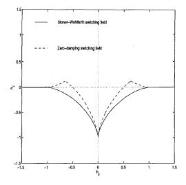
Fig. 1. For slowly applied field pulses, or large damping, Stoner-Wohlfarth analysis predicts magnetization reversal only for normalized applied fields below the solid curve. For an instantly applied field pulse and zero damping, magnetization reversal may occur for normalized applied fields below the dashed curve.
