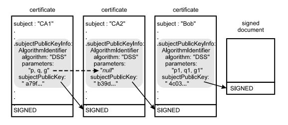
Figure 3 - Parameter Inheritance in Certification Path
