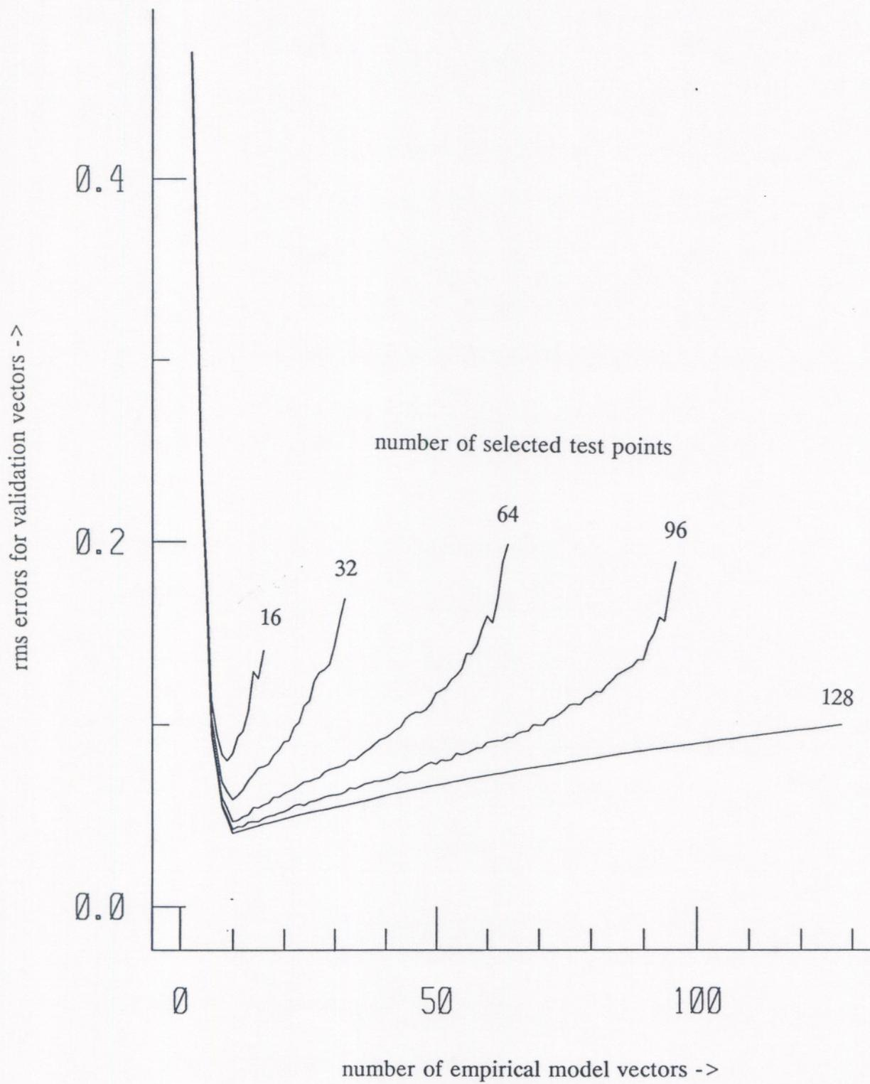
Figure 5. rms difference between predicted values and true values using SVD derived models and an rms measurement noise of 0.1
