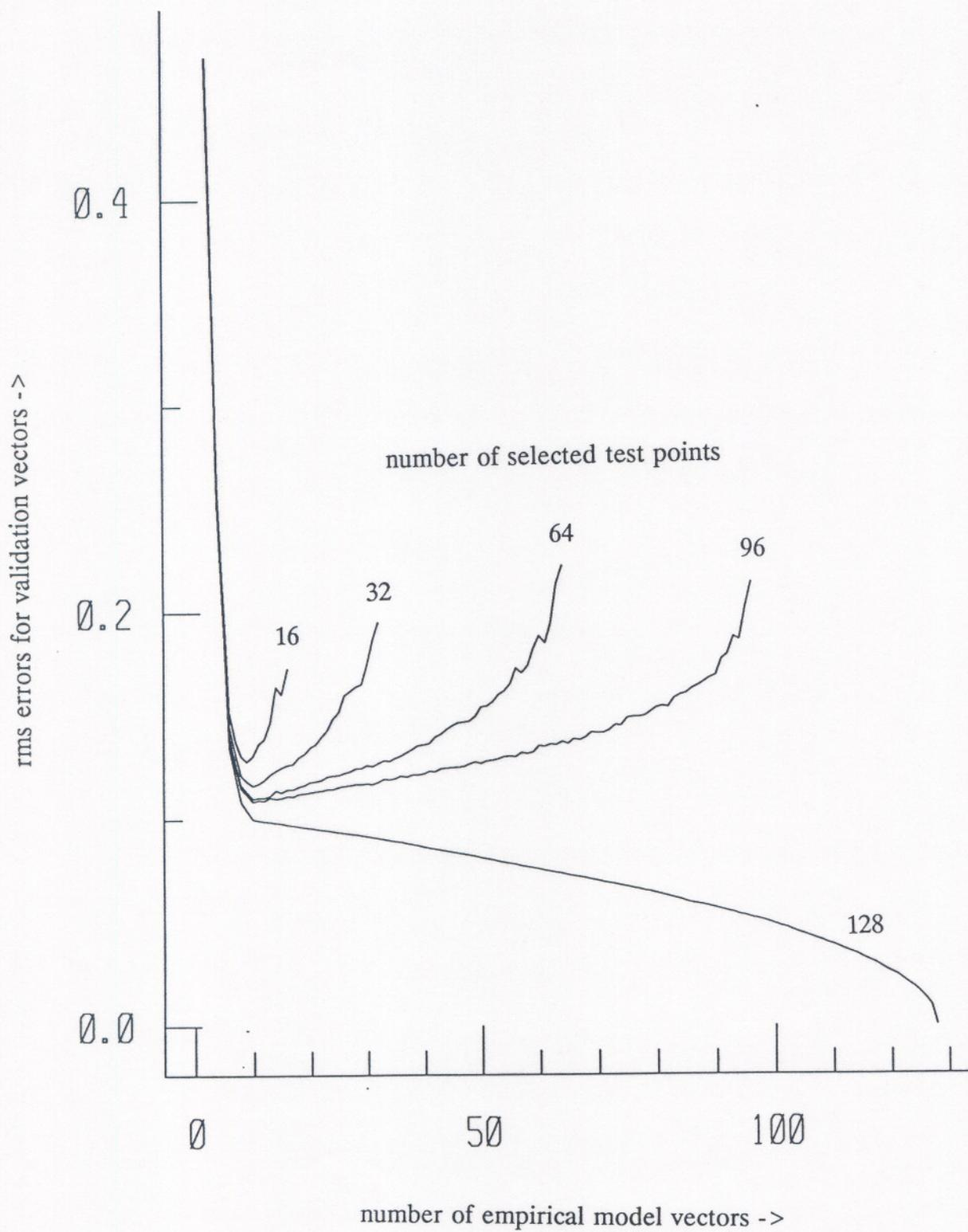
Figure 4. rms difference between predicted values and measured values using SVD derived models and an rms measurement noise of 0.1
