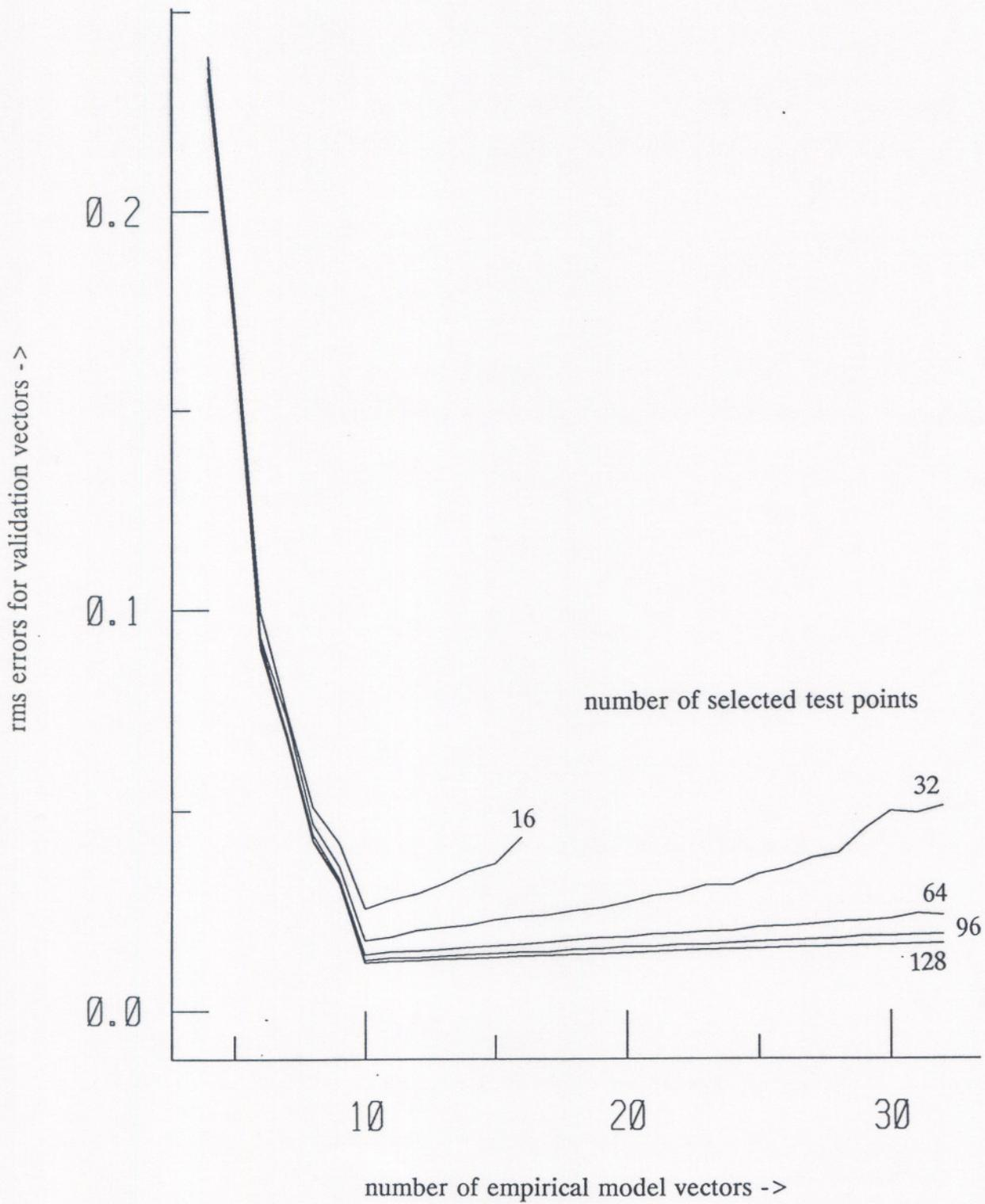
Figure 7. rms difference between predicted values and true values using SVD derived models and an rms measurement noise of 0.03
