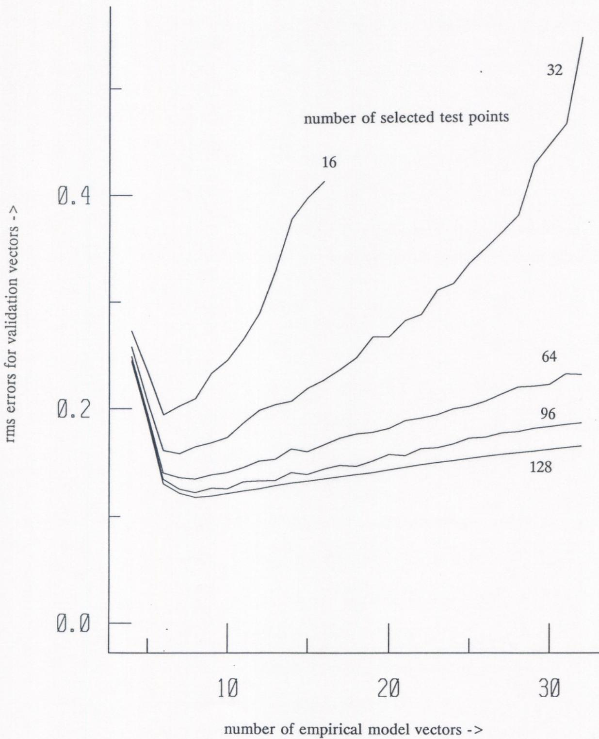
Figure 6. rms difference between predicted values and true values using SVD derived models and an rms measurement noise of 0.3
