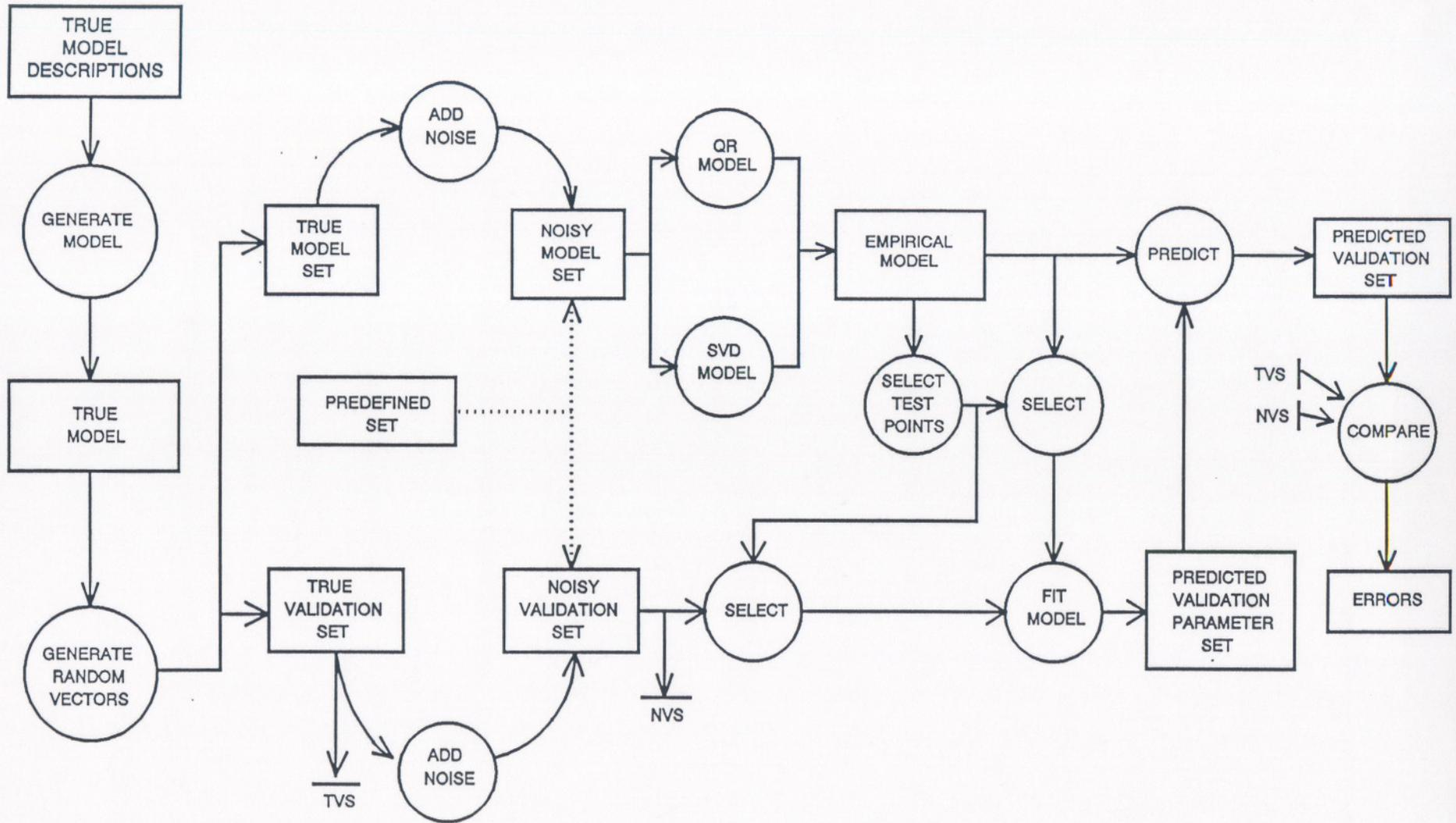
Figure 1. Block Diagram of Simulation Program
