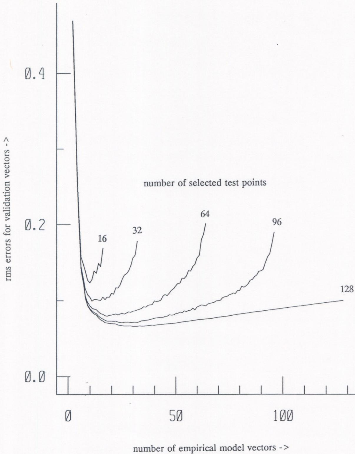
Figure 3. rms difference between predicted values and true values using QRD derived models and an rms measurement noise of 0.1
