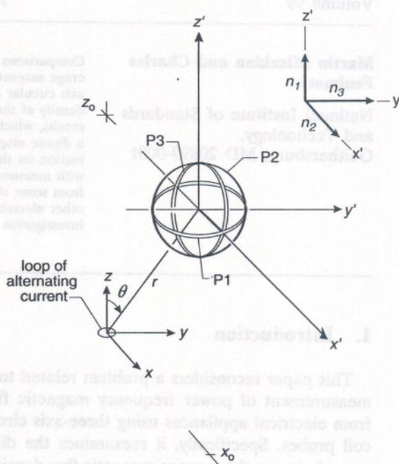
Fig. 1. Three-axis magnetic field probe with its center at  $x = x_0$ ,  $y = 0$ , and  $z = z_0$ . A small current loop producing a dipole magnetic field is located at the origin of the unprimed coordinate system. The unit vectors  $\mathbf{n}_1$ ,  $\mathbf{n}_2$ , and  $\mathbf{n}_3$  are normal to the areas of probes P1, P2, and P3, respectively. Changes in the angle  $\theta$  correspond to varying the orientation of the dipole with respect to the probe.
