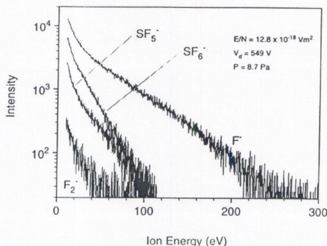
FIG. 2. Ion flux energy distributions for negative ions sampled from a Townsend discharge in sulfur hexafluoride.
