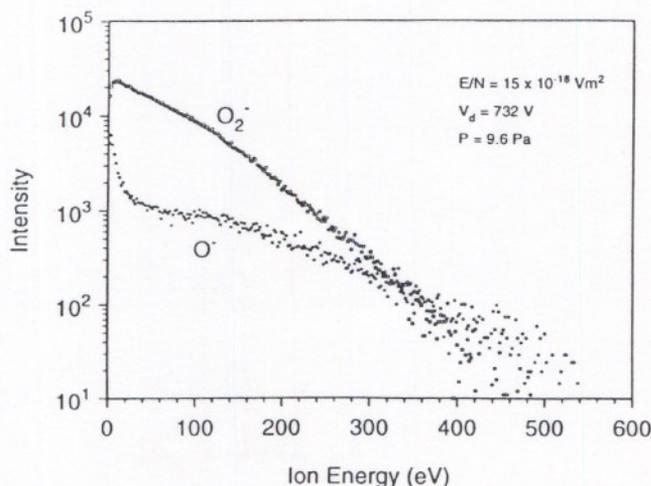
FIG. 1. Ion-flux energy distributions for negative ions sampled from a Townsend discharge in oxygen.
