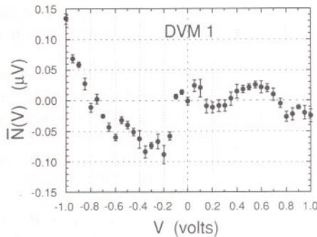
Fig. 2.  $\bar{N}(V)$  versus  $V$  curve for DVM1. The  $N(V)$  are the deviations in  $\mu\text{V}$  from the linear least-squares fit to the  $C(V)$  versus  $V$  data, as given by (7). The  $\bar{N}(V)$  are the averages obtained from six different Josephson array calibration runs.
