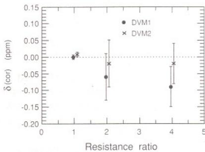
Fig. 3.  $\delta(\text{cor}) = \bar{a}_{\text{DVM}}(\text{cor}) - \bar{a}_{\text{POT}}$  results for 1:1, 2:1, and 4:1 resistance ratios using DVM1 and DVM2.  $\delta(\text{cor})$  would be zero for exact agreement between the DVM and potentiometric methods. The data for DVM1 and DVM2 are slightly displaced for clarity.
