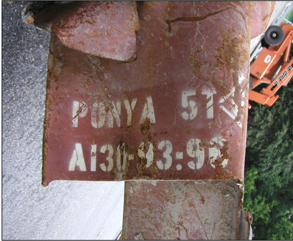
Figure 2. Characteristic stenciling found on the lower portions of the perimeter column panels. Markings indicate this piece was in WTC 1 (“A”), column number 130, spanning floors 93-96 (colored orange in Figures 3 and 4): this is the panel hit by the nose of the first aircraft. (NIST)
