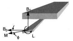
FIG. 1. Experimental configuration: A cantilever experiences a torque *L* when the magnetization *M* of the deposited magnetic film is aligned with the applied field  $B_0$  and an additional torque field  $B_T$  is present. For small values of the cantilever twist angle  $\phi$ , the torque is proportional to  $\phi$ .
