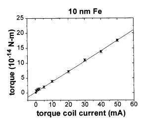
FIG. 3. Torque vs torque coil current for an iron film thickness of 10 nm.
