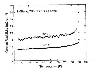
FIG. 3. Temperature dependence of specific contact resistivity  $\rho_{c}$  showing only a 25% rise in  $\rho_{c}$  of high-quality *in situ* contacts from 4 to 90 K.
