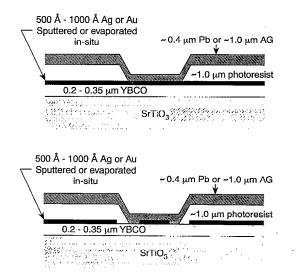
FIG. 1. Contact test geometries: (a) Window made in photoresist insulating layer with replaceable counter electrode of Pb or Ag. (b) Patterned *in situ* contact pad within photoresist window to eliminate spreading conductance into the surrounding *in situ* noble metal region (shown as black region in figure).
