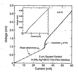
FIG. 2. Voltage vs current characteristic of  $2 \times 2 \mu m^2$  in situ Ag/YBCO contact showing 0.4 mA supercurrent (insert) and extensive ohmic region to more than 30 mA (>10<sup>6</sup> A/cm<sup>2</sup> transport current density through contact) before reaching the  $J_c$  of the Pb counterelectrode. Values of the specific contact resistivity  $\rho_c$  given in Table I were determined from this extensive linear region.
