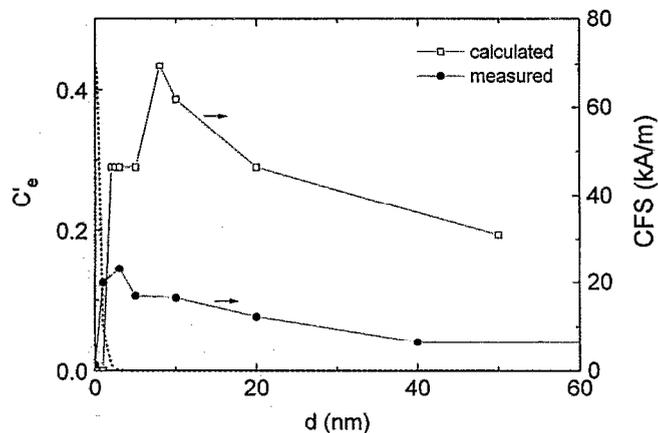
FIG. 2. Calculated and measured coercive force splitting as a function of interlayer separation  $d$ . The dotted curve on the left of the diagram represents the variation of  $C_e'$  with  $d$ .
