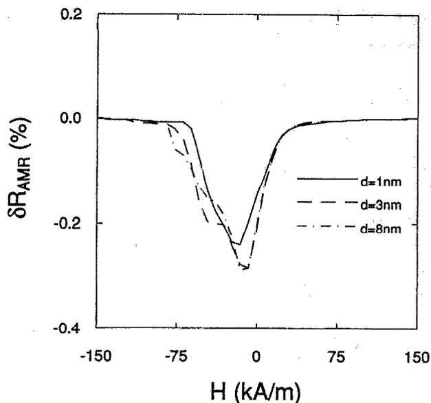
FIG. 3. Calculated AMR as a function of  $H$  for interlayer separations of 1, 3, and 8 nm ( $H$  is parallel to  $J$ ).
