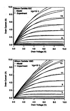
Fig. 7. Silicon carbide MOSFET simulated (dashed) and measured (solid) output characteristics as a function of gate voltage for (a) 25 °C and (b) 100 °C.
