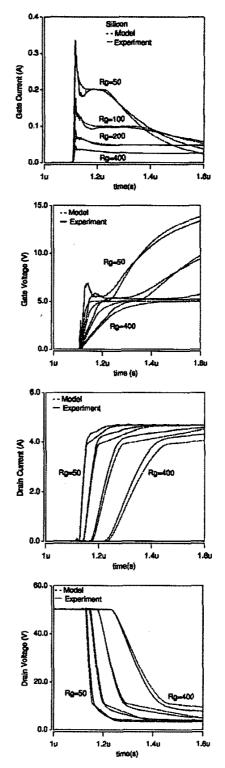
Fig. 9. Silicon carbide MOSFET simulated (dashed) and measured (solid) turn-on waveforms as a function of gate resistance: (a) gate current, (b) gate voltage, (c) drain current, and (d) drain voltage.
