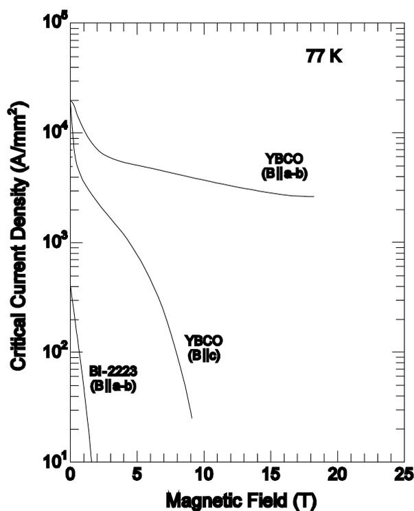
**Figure 3.** Critical-current density as a function of magnetic field for high- $T_c$  superconductors at liquid-nitrogen temperature (from a compilation by Lee<sup>8</sup>). The critical-current density  $J_c$  is referenced to the superconductor area alone.
