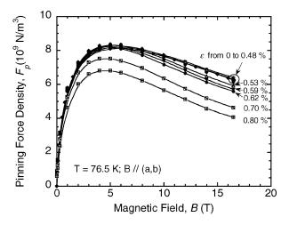
Fig. 5. Pinning force density as a function of magnetic field at 76.5 K for a Cu-laminated YBCO coated conductor for various values of axial tensile strain up to 0.8%.
