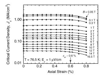
Fig. 2. An overview of  $J_c(B, \varepsilon)$  data obtained at 76.5 K on a Cu-laminated YBCO coated conductor. Measurements were performed over a wide range of magnetic field (from 0.05 T to 16.5 T) and axial tensile strain (up to 0.8%). Magnetic field was applied parallel to the YBCO (a, b) plane and perpendicular to the current-flow direction.
