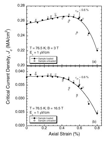
Fig. 3. Critical-current density as a function of axial tensile strain at 76.5 K for a Cu-laminated YBCO coated conductor, in magnetic fields of (a) 3 T and (b) 16.5 T, applied parallel to the YBCO (a, b) plane. Data when the sample was loaded and unloaded are respectively labeled by corresponding unprimed and primed letters. The irreversible strain limit  $\varepsilon_{irr}$  is about 0.6%, mostly independent of magnetic field.
