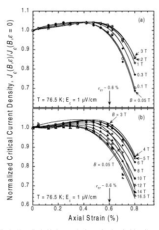
Fig. 4. Normalized critical-current density as a function of axial tensile strain at 76.5 K for a Cu-laminated YBCO coated conductor, both in low (0.05 T to 3 T) and high (3 T to 16.5 T) magnetic fields.  $J_c$  degradation unexpectedly shrinks with magnetic field from 0.05 T to about 2–3 T. Above 3 T, the reverse occurs as this degradation grows systematically with increasing field up to 16.5 T, where it reaches its maximum.
