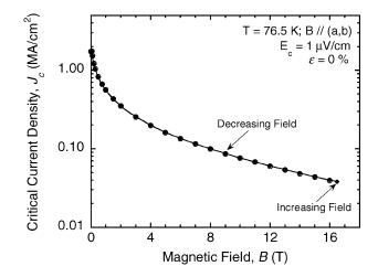
Fig. 1. Critical-current density as a function of magnetic field at 76.5 K and zero applied strain for a Cu-laminated YBCO coated conductor. Magnetic field was applied parallel to the YBCO (a, b) plane and perpendicular to the current-flow direction.
