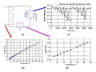
Figure 3. Gas-sensor SoC-calibration requirements.
