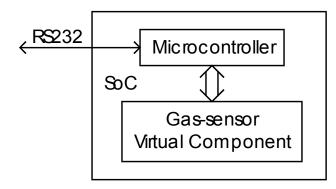
Figure 1. Gas-sensor SoC system architecture.
