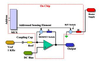
**Figure 7.** A schematic diagram of the gas-sensor calibration and characterization.
