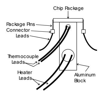
Figure 4. Microhotplate temperature-sensor calibration.
