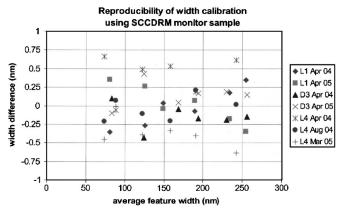
FIG. 3. Reproducibility of linewidth measurements on three SCCDRM chips: K143 L4, K147 L1, and K143 D3. All widths are measured relative to the SCCDRM monitor sample, indicating that a realization of tip width relative to the SI meter can be accomplished with a standard uncertainty of 1 nm or less.
