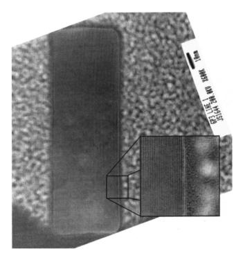
FIG. 1. Negative of the high-magnification (400 k $\times$ ) HRTEM image of the narrowest feature used. At this magnification, the silicon lattice fringes are visible as can be seen in the enlarged portion of the sidewall shown in the inset.
