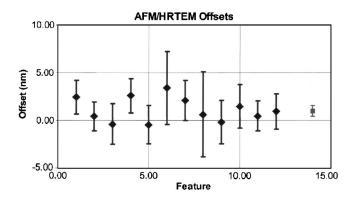
FIG. 2. Comparison of the individually estimated AFM offsets and the weighted-mean offset. The uncertainties shown in the plot are the expanded uncertainties (k=2). The uncertainties include the reproducibility of both the HRTEM and AFM results and the influence of relative positioning uncertainty. The weighted average and expanded uncertainty (k=2) are 1.03 nm±0.58 nm.
