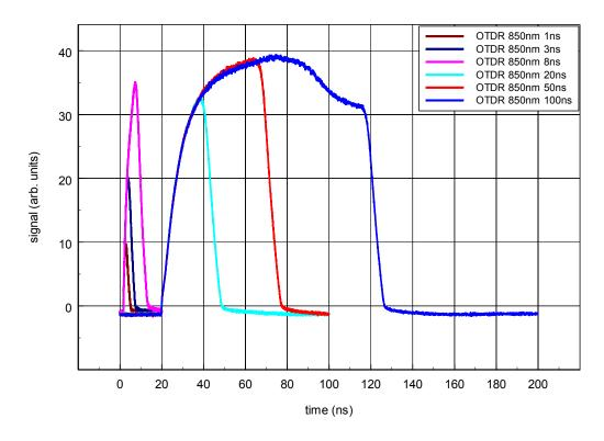
Figure 2. OTDR output at 850 nm, available pulse widths.
