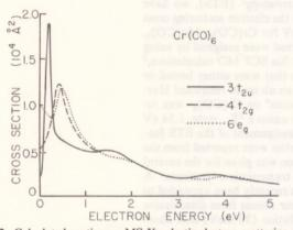
Figure 2. Calculated continuum MS-X $\alpha$  elastic electron scattering cross section vs. electron energy for Cr(CO)<sub>6</sub> for three different potentials obtained by adding 0.5 electrons to the  $3t_{2u}$ ,  $4t_{2g}$ , and  $6e_g$  orbitals, respectively.
