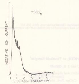
Figure 1. Ion current vs. electron impact energy on  $Cr(CO)_6$ . The ions are essentially all  $Cr(CO)_5^-$ .
