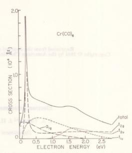
Figure 3. Decomposition of calculated cross section by symmetry of continuum electron for the scattering potential given by occupation of the  $3t_{2u}$  orbital (eg and  $t_{1g}$  channels give  $\sigma < 30$  Å<sup>2</sup> and are not shown).
