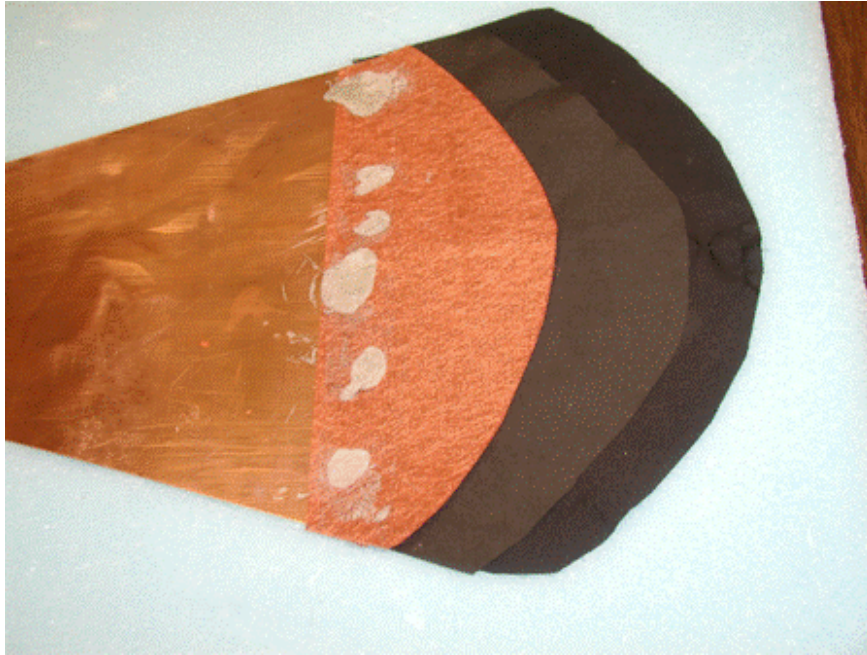
Figure 35. Close-up of the “layered-moon” resistive termination.
