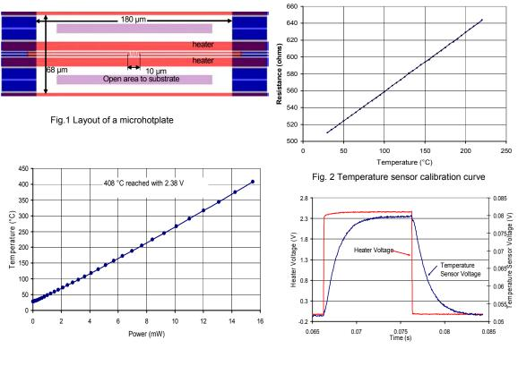
Fig. 3 Microhotplate power efficiency
