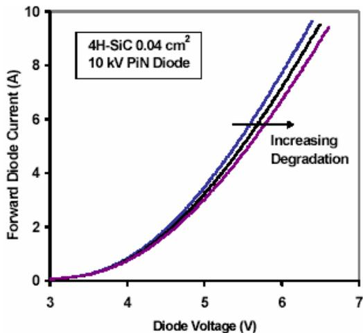
Figure 4. On-state characteristics of a high-voltage SiC PiN diode after various levels of forward bias stress.
