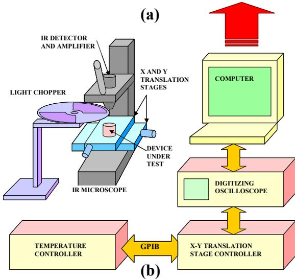
Figure 3. Transient Thermal Current Uniformity Degradation System: (a) front panel user interface, (b) experimental setup.
