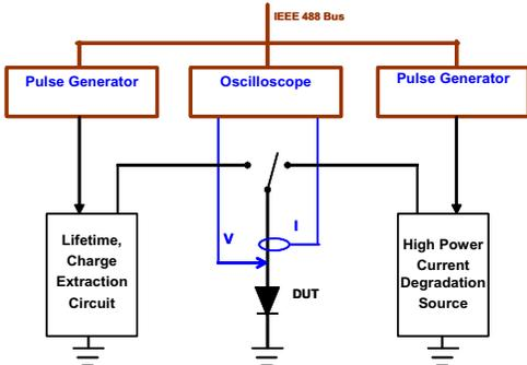
Figure 1. Pulsed Degradation and Monitoring System.
