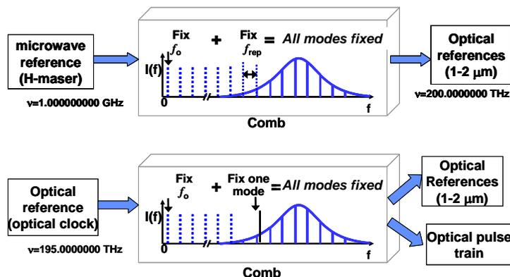
Fig.1. Schematic of the basic operation of a frequency comb. The comb can be referenced to either an rf or optical reference. In either case, its purpose is to faithfully translate the stability and coherence of the reference source across the optical spectrum.
