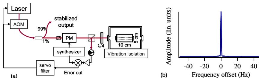
Figure 2: (a) Pound-Drever-Hall lock of the laser to the ULE optical cavity. (b) The resulting linewidth of the stabilized laser, measured by recording 1.5 seconds of the beat note between this laser and a narrow-linewidth fiber frequency comb (described in the next section), and then Fourier transforming the signal. The linewidth shown here is 1 Hz, as measured from the 1.5 seconds of data.
