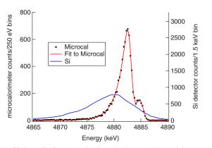
FIG. 2. (Color online) Measured microcalorimeter alpha particle spectrum from  $^{209}$ Po (black), a fit to the data (red), and the same source measured with a Si detector (blue).
