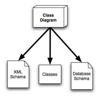
Fig. 2 UML Class diagram generates code
