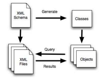
Fig. 3 Relationship between XML schema, classes and XML instances
