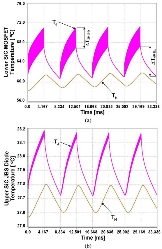
Fig. 3: Temperature waveforms at the SiC-chip surface ( $T_j$ ) and chip-package interface ( $T_h$ ) for the lower SiC MOSFET (SiC\_MOS1) and the upper SiC JBS diode (SiC\_JBS2) in the 100 A, 10 kV half-bridge SiC MOSFET/JBS power module shown in Fig. 2.
