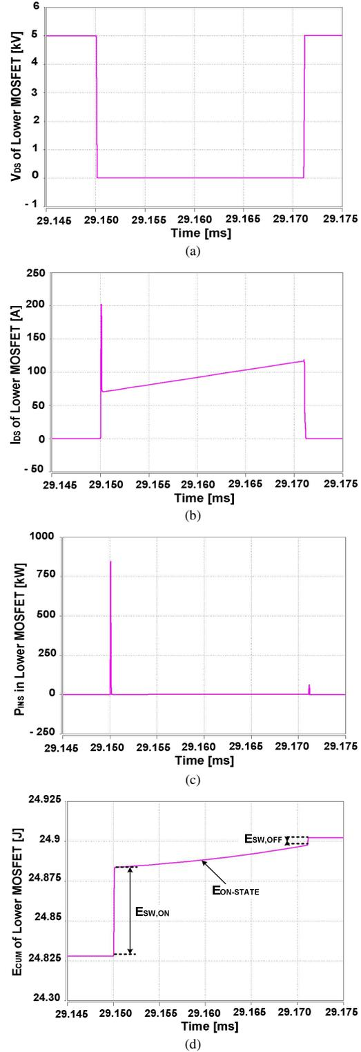
**Fig. 5:** One switching cycle from the 20 kHz simulation of the (a) drain-to-source voltage ( $V_{DS}$ ), (b) drain current ( $I_{DS}$ ), (c) instantaneous dissipated power ( $P_{INS}$ ), and (d) cumulative dissipated energy ( $E_{CUM}$ ) for the active lower SiC MOSFET (SiC\_MOS1) in the 100 A, 10 kV half-bridge SiC MOSFET/JBS power module previously shown in Fig. 2.
