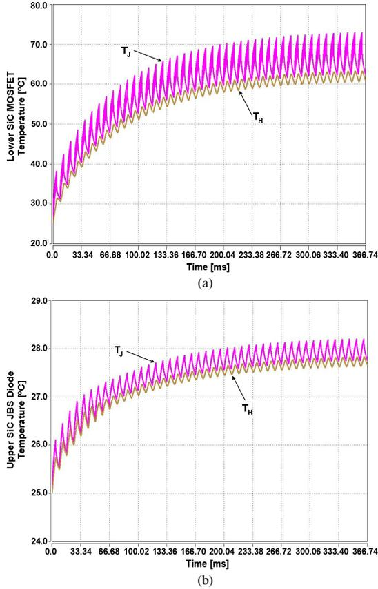
**Fig. 4:** Simulated thermal response at startup for the average power dissipated in the SiC\_MOS1 (a) and SiC\_JBS2 (b) indicating the temperature at the junction ( $T_J$ ) and chip-package interface ( $T_H$ ).
