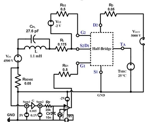
**Fig. 1:** The basic 5 kV boost converter used for the 100 A, 10 kV half-bridge SiC MOSFET/JBS power module simulation.
