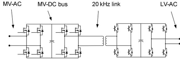
Fig. 7: Example of a building block circuit for an SSPS. This building block converts medium voltage AC (MV-AC) at the primary (PRI) to low voltage AC (LV-AC) at the secondary (SEC).
