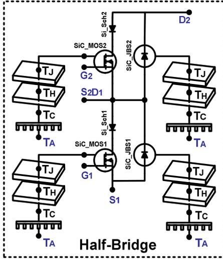
Fig. 2: Circuit topology of the 100 A, 10 kV half-bridge SiC MOSFET/JBS power module with series silicon Schottky power diodes to prevent reverse conduction in the SiC MOSFETs.
