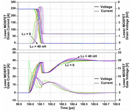
Fig. 6: The effect of the gate inductance on the drain-source voltage, drain current, gate-source voltage, and gate current waveforms for five different values of the gate inductance  $L_G$  (0 H, 10 nH, 20 nH, 30 nH, 40 nH) for the lower SiC MOSFET in the 100 A, 10 kV half-bridge power module.
