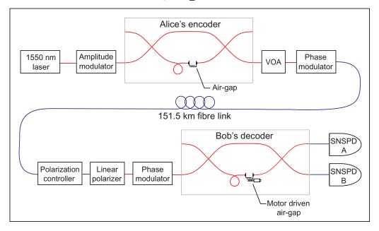
**Figure 1.** Optical train of the phase-encoding QKD system used in this work. The variable optical attenuator (VOA) provides attenuation to the single-photon level, from which the amplitude modulator provides the different  $\mu_j$  levels needed for the decoy level protocol. Red lines indicate polarization maintaining fibre, and blue lines represent single-mode fibre. Photons are detected by two SNSPDs biased to yield matching detection efficiencies.
