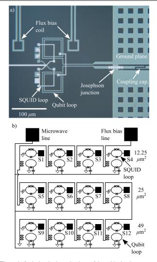
Figure 1. Optical and schematic views of the qubit circuit.
