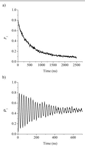
**Figure 3.** Low-temperature (T = 20 mK) measurements for the qubit with a c-Al<sub>2</sub>O<sub>3</sub> tunnel barrier. (a) Energy relaxation time  $T_1 = 500 \text{ ns.}$  Measurement fidelity = 80%. (b) Rabi oscillations: dephasing time  $T_2 \sim 140 \text{ ns.}$  Rabi visibility = 70%.
