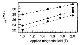
Fig. 4. Dots show critical currents  $I_{crit}$  from Fig. 3(a) versus applied magnetic field. Resistance features in Fig. 3 can be assigned to three critical currents that shift linearly with field. Dashed lines are linear fits for each set.
