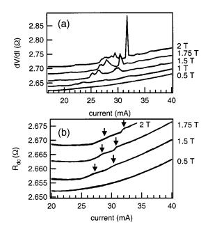
Fig. 3. (a) dV/dI versus dc current at T = 4 K for 250 ×80-nm diameter elliptical CPP spin-valve. Data at different magnetic fields are vertically offset for clarity. dV/dI spike positions give critical currents  $I_{crit}$ . (b) DC resistance at T = 4 K measured simultaneously for the same device. Arrows mark critical currents  $I_{crit}$  corresponding to dV/dI spikes in (a).
