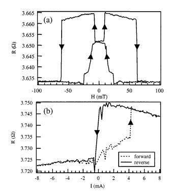
Fig. 2. (a) Room-temperature resistance measured with lock-in amplifier with 0 dc current versus in-plane magnetic field for 80-nm-diameter circular CPP Co–Cu–Co spin-valve shows field-induced GMR. (b) Room-temperature dc resistance versus dc current for same device as in (a) shows current-induced hysteretic switching. Current sweeps from negative to positive (forward, dashed line) and from positive to negative (reverse, solid line).
