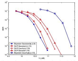
**Fig. 1.** Performance in  $S(\alpha = 2)S$  (Gaussian) noise (side info. required by each metric, and equations, indicated in ()'s in legend)
