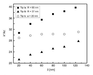
Fig. 6. Normalized contact stiffness  $k^*/k_c$  as a function of cantilever deflection  $\delta$ . The three sets of data were obtained with three different tips attached to cantilevers with nearly identical values of their spring constants  $k_c$ . The differences in the values of  $k^*/k_c$  were caused by the differences in tip geometry.
