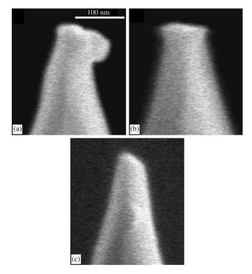
Fig. 3. SEM images of three tips affected by fracture in the AFAM measurements. The images were acquired after the (a) third, (b) fifth, and (c) first AFAM tests. The scale is the same for all three images.
