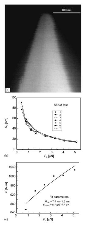
Fig. 5. (a) SEM image of new tip IId. (b) Tip radius  $R_{\rm H}$  versus applied static load  $F_{\rm C}$  calculated using the Hertzian contact model. (c) Comparison between experimental values for  $k^*$  (points) and those predicted using the DMT contact-mechanics model as defined in Eq. (3) (line). The values for R and  $F_{\rm ad}$  used as fit parameters are given.
