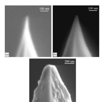
Fig. 2. SEM images of brand new tips revealing the wide differences in possible new-tip geometry. The scale is the same for all three images. (a) Sharp tip with radius of curvature R < 10 nm.(b) Tip with  $R \sim 20 \text{ nm. (c)}$  Very blunt tip with possible surface contamination not seen in other tips.
