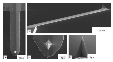
Fig. 1. SEM images of one of the AFM cantilevers used in this study. (a) Plan view and (b) side view images used to measure the cantilever dimensions. (c) Close-up of the region containing the tip. Note that the tip is not located at the exact end of the cantilever, and that the last  $20-25 \,\mu\text{m}$  of the cantilever's length has a different geometry. (d) Side view of the AFM tip.
