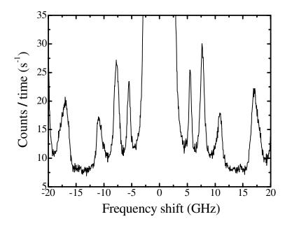
**Figure 2**. BLS spectrum with an angle of 70° between the substrate normal and the incident beam. Ordinates are the counts per unit time in one channel of the multichannel analyzer.
