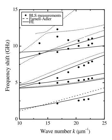
**Figure 3**. BLS measurements. Farnell-Adler calculations and FE calculations with  $v_1 = 2784$  m/s,  $v_2 = 1354$  m/s,  $\rho = 1187$  kg/m<sup>3</sup>, h = 140 nm, and w = 65 nm.
