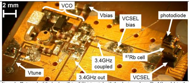
Figure 1. Photograph of the local oscillator (LO) integrated with the physics package. The LO modulates the vertical-cavity surface-emitting laser (VCSEL) at 3.4173 GHz, exciting the coherent-population-trapping (CPT) resonance of gaseous <sup>87</sup>Rb atoms contained in a glass and silicon cell. The photodetector at the top of the physics package receives the laser light and control electronics (not shown) tune the LO to a lock on the CPT resonance.
