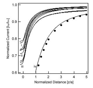
**Fig. 3.** Approach curves to 20 wt% (i), 40 wt% (ii), and 60 wt% (iii) PEG 3000 hydrogel surfaces. For each hydrogel, three separate locations were sampled and plotted. In the fourth curve (iv) simulated currents for approach to an impermeable insulator are compared with experimental data for approach to a glass surface. Simulated data (filled circles) were calculated with the analytical approximation of Amphlett and Denault [30] for  $R_g = 5.09$ .
