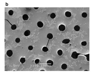
**Fig. 5.** SECM image of hydrated, 40 wt% PEG 508 hydrogel photopolymerized around a sphere template that has been dissolved (a) and SEM image of the same hydrogel (different region) after vacuum drying (b).
