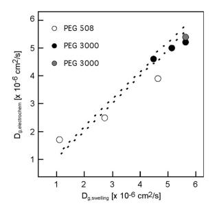
**Fig. 4.** Comparison of  $D_g$  estimated electrochemically vs.  $D_g$  predicted by equilibrium swelling. Pearson's linear correlation coefficient is 0.98. Dashed lines indicate the range of predicted values. Open circles are PEG 508 gels; filled circles are PEG 3000 gels. Gray circle is a 20 wt% PEG 3000 hydrogel from a different PEGDA synthesis.
