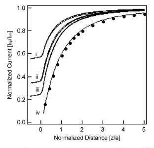
**Fig. 2.** Approach curves to 20 wt% (i), 40 wt% (ii), and 60 wt% (iii) PEG 508 hydrogel surfaces. For each hydrogel, three separate locations were sampled and plotted. In the fourth curve (iv) simulated currents for approach to an impermeable insulator are compared with experimental data for approach to a glass surface. Simulated data (filled circles) were calculated with the analytical approximation of Amphlett and Denault [30] for  $R_g = 5.09$ .
