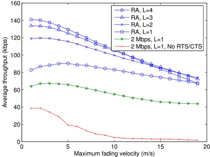
Fig. 5. FTP throughput on  $8 \times 8$  grid with Rayleigh fading (RA = rate adaptation)
