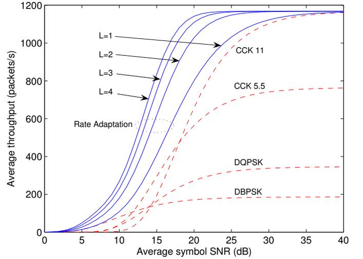
Fig. 3. Link throughput vs. average SNR in quasi-static Rayleigh fading
