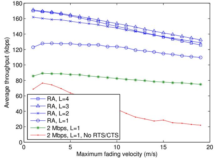
Fig. 6. FTP throughput on  $8 \times 8$  grid with Ricean fading ( $K = 5$  dB)
