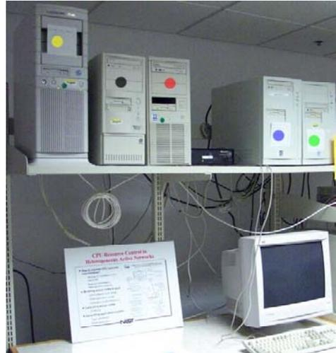
**Fig. 5.** The five-node active-network test bed we set up in our laboratory at NIST in order to conduct our experiments and to make measurements. The nodes from left to right: Yellow, Black, Red, Blue, and Green.
