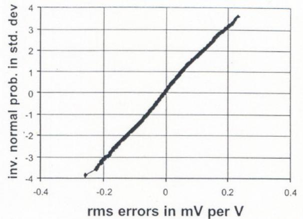
Fig. 6. RMS measurement error for CSL quantization is normally distributed and much smaller than errors shown in figs. 2 and 4.
