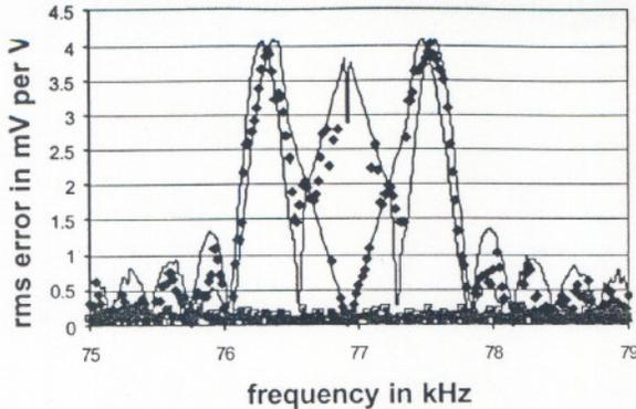
Figure 7. Predicted rms error range for ramp quantization (maximum-upper solid line, minimum-lower solid line) and measurement rms error for ramp quantization (dark diamonds), and for CSL quantization (gray squares).
