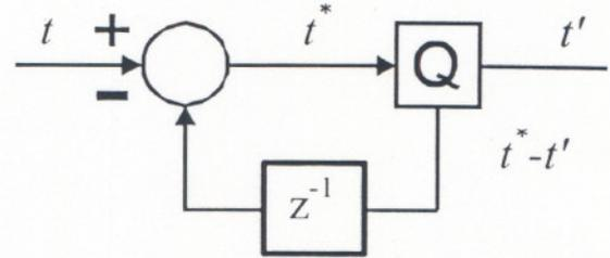
Fig. 5. Cumulative sum limited quantizer; the quantization error from quantizer Q is fed back to an adder via a unit sample delay to limit the cumulative sum of quantization errors.
