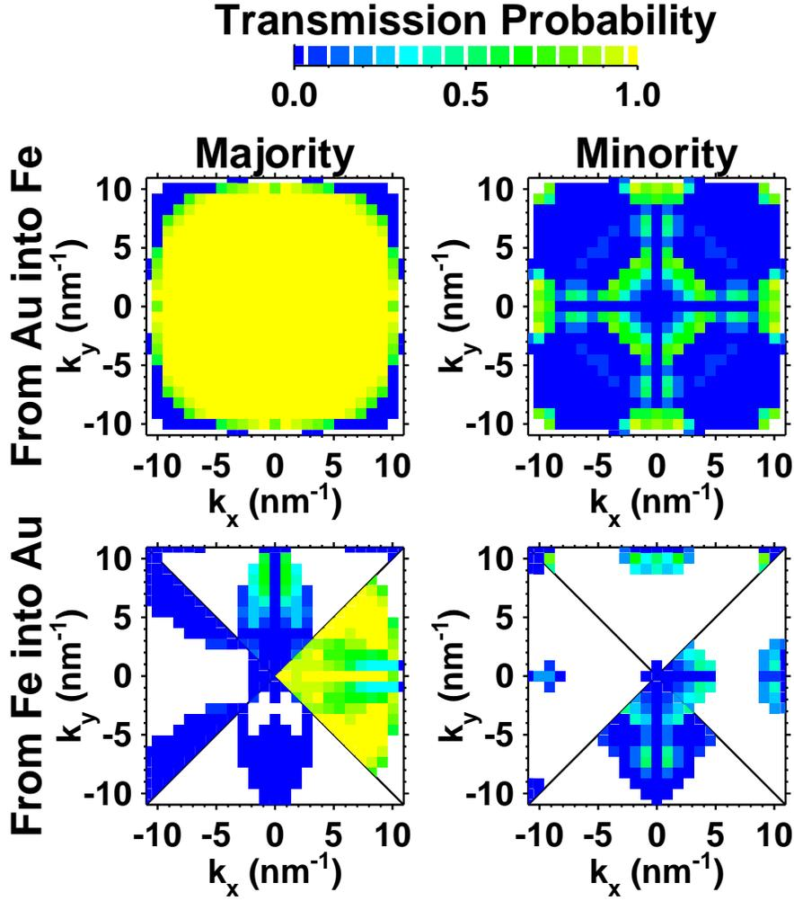
FIG. 1. Spin-dependent transmission probabilities for Au/Fe(001). The transmission probabilities are shown for various points on the Fermi surface projected onto the interface Brillouin zone. The color scale for the transmission probability is at the top. The top (bottom) two panels show the transmission for electrons incident from the Au (Fe) into the Fe (Au). The two right (left) panels show the transmission probabilities for the minority (majority) electrons.
