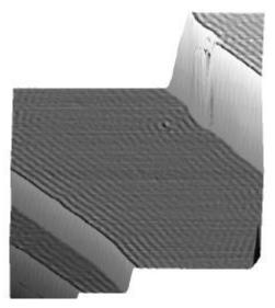
Fig. 2: STM image, 50x50nm, of the Cu(111) surface obtained at 4.3 K showing constructive interference produced by the scattering of the 2D surface state from step edges and defects.
