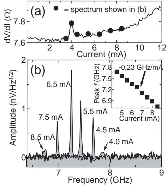
**Fig. 5.** Precession. (a) Differential resistance  $dV/dI$  vs. current  $I$  for  $\mu_0 H = 0.1T$  along the in-plane easy axis. (b) High frequency spectra taken at several different values of current through the device, corresponding to the symbols in (a). Variation of frequency  $f$  with current (inset). Used by permission from Rippard et al. [30]
