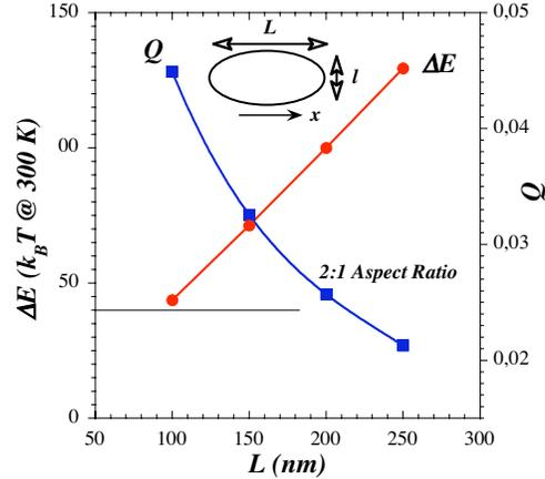
**Fig. 18.** Energy barrier between long and short axis uniformly magnetized elliptical elements ( $\text{Ni}_{80}\text{Fe}_{20}$ ,  $d = 2.5$  nm; room temperature,  $T_R = 300$  K). The shape induced anisotropy  $Q = 2K/(\mu_0 M_S^2) = H_K/M_S$  is also plotted.
