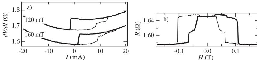
**Fig. 3.** Differential resistance. (a)  $dV/dI$  of a pillar device exhibits hysteretic jumps as the current is swept. The current sweeps begin at zero; light and dark lines indicate increasing and decreasing current, respectively. The traces lie on top of one another at high bias, so the 120.0 mT trace has been offset vertically. (b) Zero-bias magnetoresistive hysteresis loop for the same sample. Used by permission from Katine et al. [8]
