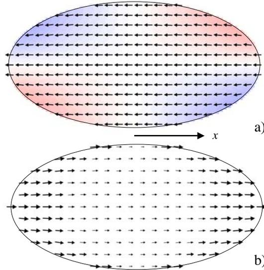
**Fig. 17.** Magnetization (a) and effective field (b) distributions typical of flat elliptical elements with long axis in the 130 nm range and 2:1 aspect ratio.  $\text{Ni}_{80}\text{Fe}_{20}$ , thickness  $d = 2.5$  nm.
