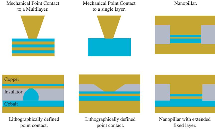
**Fig. 1.** Schematic experimental geometries. In each geometry, copper layers are tan, cobalt layers are blue, and insulating layers are gray, as labeled in the lower left panel. Other ferromagnetic materials may be substituted for Co and non-magnetic materials for Cu.
