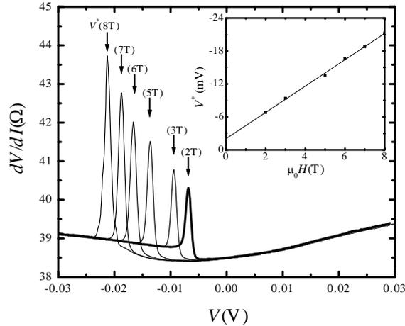
**Fig. 2.** Differential resistance of a mechanical point contact as a function of current for various applied magnetic fields. The peak in differential resistance that occurs for only one current direction indicates a spin transfer effect. The inset shows that the current at the peak in the differential resistance increases linearly with the applied field. Used by permission from Tsoi et al. [4].
