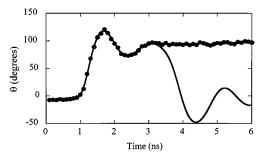
Fig. 2. Magnetization rotation angle as a function of time of a easy axis-biased Permalloy film subjected to a 2.0 ns magnetic field pulse. The easy axis bias field is 80 A/m. The measurement utilized the SH-MOKE technique. The pulse amplitude of 1.04 kA/m is applied along the hard axis. The solid line is the Landau-Lifshitz-Gilbert simulation result.
