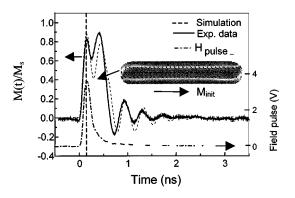
Fig. 1. The GMR response and simulated transverse magnetization ( $\alpha = 0.02$ ) for a  $0.8 \,\mu$ m × 4.8  $\mu$ m spin valve subjected to 0.15 ns, 6.4 kA/m transverse field pulse. The dashed-dot line represents the applied magnetic field pulse. The inset shows a micromagnetic simulation of the magnetization state at 0.31 ns after the onset of the transverse field pulse.
