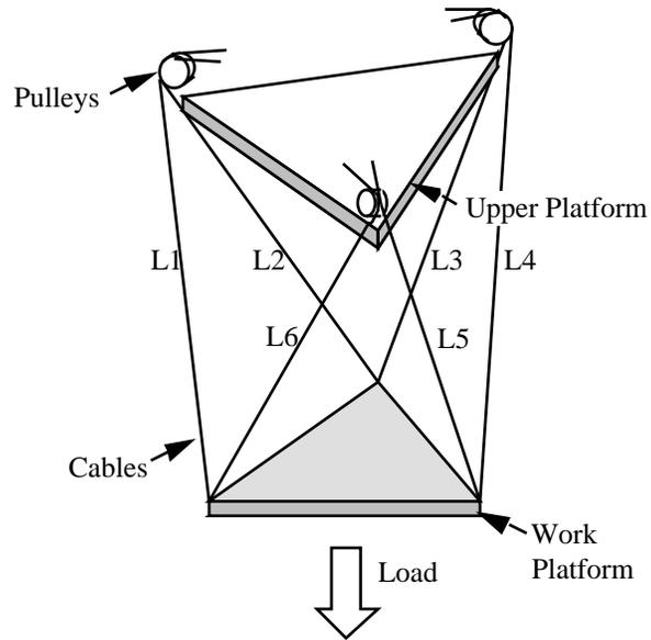
Figure 1 - Basic Concept of Stewart Platform Parallel Link Manipulator using cables as parallel links.
