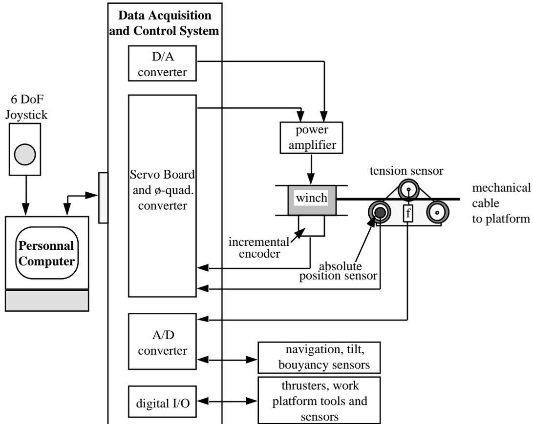
Figure 4 - Block Diagram showing One of Six Channels of the S3P Control System
