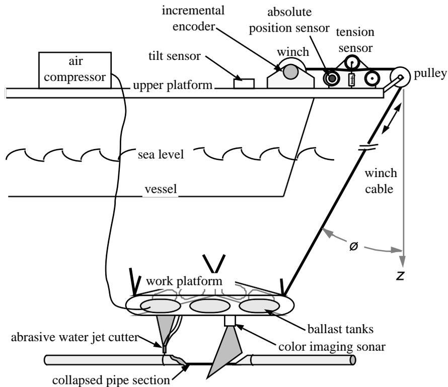
Figure 3 - Component diagram of the S3P showing one of six cables/channels and applying the S3P to underwater pipeline inspection and repair.
